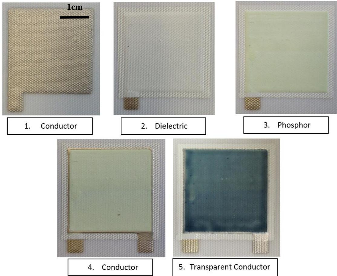
*Figure 4. The print process showing the layer by layer deposition of inks to form the EL lamp.*
