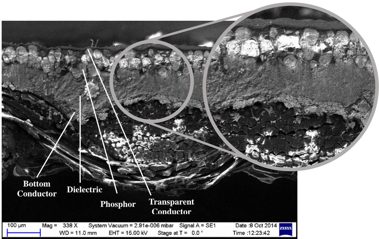
*Figure 5. SEM image showing distinct dispenser printed layers - total layer thickness 307μm.*
