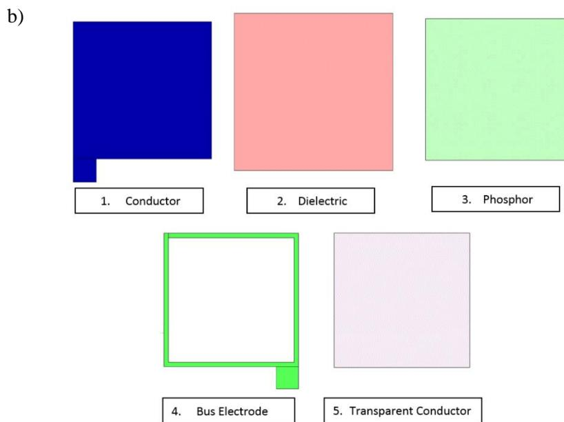
**Figure 2.** Screen design for an EL lamp with an emitting area of 30 x 30 mm, a) full design showing all screens and sizes, b) individual screen designs.
