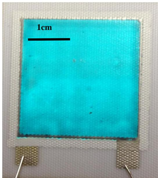
*Figure 3. A powered dispenser printed EL lamp – driven at 180 Vac, 400Hz.*
