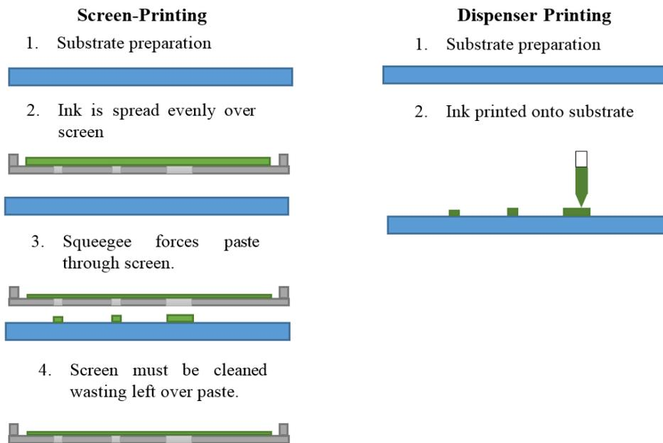
**Figure 1.** Comparison of printing process for screen-printing (left) and dispenser printing (right).
